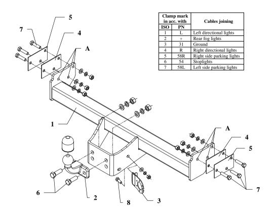
This towing hitch is designed to assembly in following cars: NISSAN TERRANO II, 3/5 doors, produced since 1993 till 2007, FORD MAVERICK, 3/5 doors, produced since 1993 till 2001 catalogue no. V18 and is prepared to tow trailers max total weight 3000 kg and max vertical mass 100 kg.
